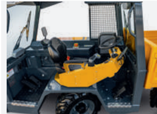
Rotating driver's platform for additional safety
